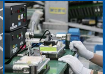
Air Leak Test
