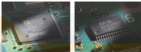
<DSP unit> ADSP-21369 Internal clock speed: 333MHz 32-bit floating point DSP Max. performance: 2000MFLOPS
