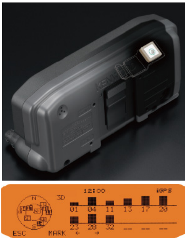
Fig. 3-4 Internal GPS Unit and GPS Satellite Information Display
