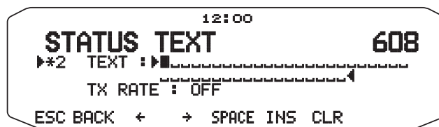
Fig. 2-12 Menu 608 (APRS - STATUS TEXT - TEXT)
