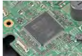
For band scope ADSP-21363 clock @333 MHz
