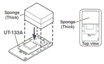
5) Attach the UT-133A to the connector on the PCB.
