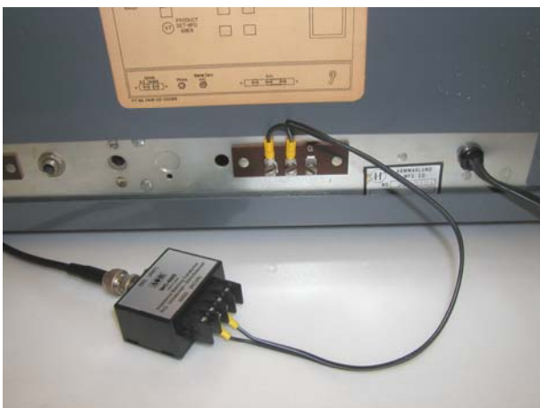
Photo shows typical classic radio (antique radio) installation with supplied twin-lead cable.
