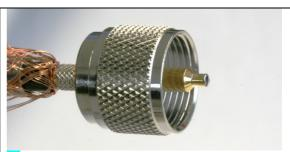
**4.** Solder the inner conductor and the inner pin at the tip.
