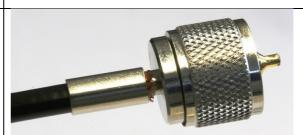
**5.** Cut off the copper braid with a side cutter and move the crimp jacket to the front.
